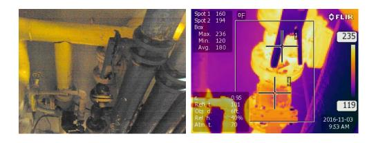
Low Pressure Steam Valve and StrainerOperating Temperature, \*F±235°Ambient Temperature, \*F104Insulation selectedFiberglass
